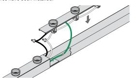
Screw LED lamps into socket.
