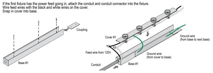
Continue run by sliding bottom of the base into the coupling and secure with appropriate screws.
