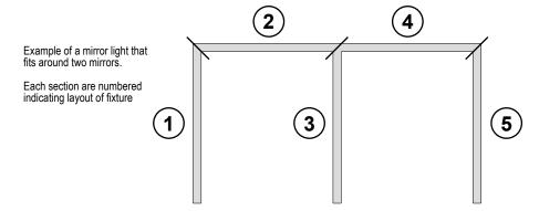
Typically the power is fed through the back of the fixture to hide any wires and conduit. Using the drawing provided, note the feed location and fixture number and drill hole through the back of fixture where the feed will be located. Step 2 The fixture can also be fed through the ends which will have 7/8 inch knock out attached. (fixture 1, 3 and 5 using example above) Remove cover and pre-drill holes every 12-15 inches apart for all of the base fixtures.
