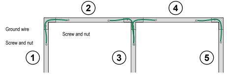
Attach the green ground wire on cover no. 1 to base no. 1. Use the same screw and nut that was used to attach the ground wires from base to Step 5 base. Each screw and nut on the base accommodates 2 sets of ground connection.
