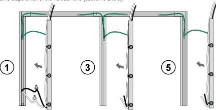
The top horizontal cover will be shipped in one piece if it is shorter than 8 feet section. Make ground connection from cover to base and wire all of the black and white wires from vertical sections (1, 3 and 5) to the cover.
