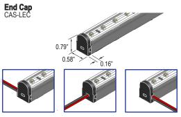
End caps include 3 openings, allowing pigtail leads to feed out of end of fixture as well as to either side of fixture.
