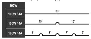
Multiple groups of modules may be daisy-chained together, so long as total length of run does not exceed 30ft.
