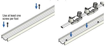
Step 2 (C) If using Linear Lens and Linear Channel; cut channel and lens to length; screw mount channel to surface; snap in lightstrip. Snap in lens after all other installation is complete.
