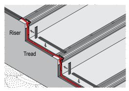
Install corner piece onto the outside corner of the step where the raceway meets the GEM-1800 step stairnose. Screw down using tapcon screw on both the riser and the tread. Install the plastic button over the tapcon crews to conseat the screws.
