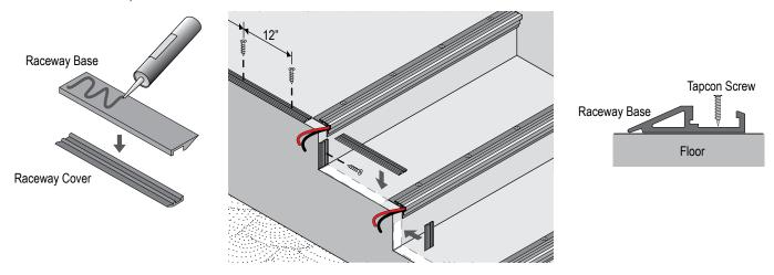
After all of the raceway bases have been installed to the tread and riser of each step, lay down the wireharness and connect the power feed from each GEM-1800 step stairnose to the main wire harness cable.
