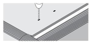
Remove the cover of the GEM-7000 housing and apply adhesive to the underside of the base. Place the GEM-7000 base back to the surface, aligning the two holes on the surface with the holes on the base and secure with tapcon screws provided.
