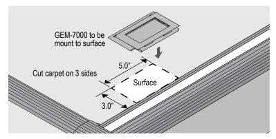
Place the GEM-7000 housing against the surface to be installed. Use the two holes on the base to mark the locations of the mounting screws. Remove the GEM-7000 housing and drill holes to the two marked spots. Use 5/32" concrete drill bit for concrete surfaces. Clean surface and remove any dust or debre.
