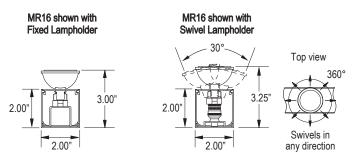
Only use GU5.3 base MR16 lamp rated for 12V, maximum 50W each. Consult lamp manufacturer for details. Lamps not included with fixture.
