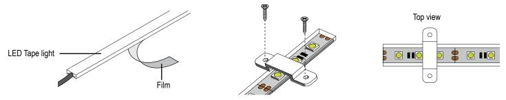
Step 5 This lightstrip runs on 24V DC. Make sure the power supply output is 24V DC. Each 20ft length consumes 86 Watts (4.3W per foot). When feeding the lightstrip, do not exceed the wattage rating of the power supply per circuit.
