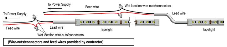
Step 3 For applications shorter than 20 feet, the lightstrip may be field-cut, in increments of approximately 4 inches (every 6 LEDs) Apply silicone or other sealant to the cut end. Do not attempt to attach connector to cut-off loose pieces of tapelight. Consult factory for custom cut lengths.
