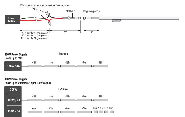
Multiple combinations of 49in and 13in fixtures may be connected together, so long as total length of run does not exceed 21ft.
