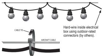
Stringlite shown mounted with no drop, to aircraft cable (by others). Ensure that aircraft cable is taut and secured. Specify cables ties. Use two cable ties per socket; one on each side.
