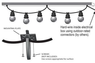
Stringlite shown mounted with drop, to aircraft cable (by others). Ensure that aircraft cable is taut and secured. Specify cable ties. Use at least one cable tie every 6 feet.
