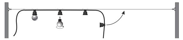
Secure junction box (by others) to surface or pole. Run 120V line voltage to junction box and hard-wire Hydra STL LED Light String inside using Step 3 outdoor rated connectors (by others)
