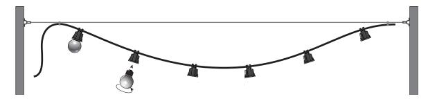
Secure junction box (by others) to surface or to pole. Run 120V line voltage to junction box and hard-wire Hydra STL LED Light String inside using Step 3 outdoor rated connectors (by others)
